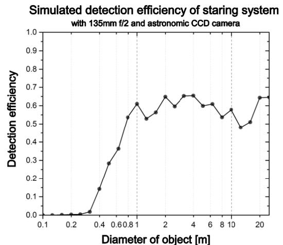
Figure 9: Simulated detection efficiency of LEO objects of the staring system as function of the object diameter.
