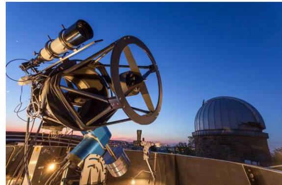
Figure 1: DLR observatory can perform passive and active optical measurements using a 17 inch telescope for imaging and single photon counting simultaneously and a 4 inch laser transmitter on an equatorial mount.
