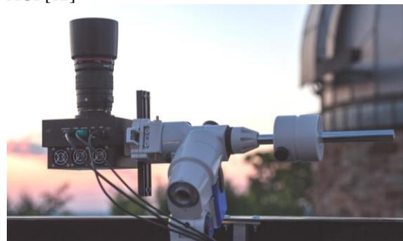
Figure 4: The staring camera system is mounted on a manual equatorial mount and records images continuously. Angular coordinates of LEO objects passing the FOV are measured which will allow rough orbit predictions.
