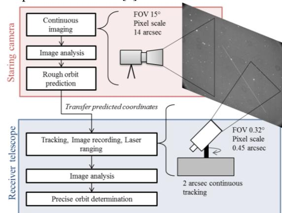
Figure 2: Layout of the proposed setup to detect unknown objects with a staring camera and send predicted coordinates to a separated system to detect the object with the receiver telescope.
