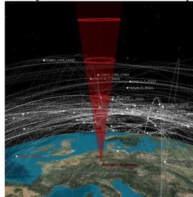
Figure 3: An illustration of satellite orbits (white lines) and the region in LEO covered by the staring cam (red cone) as it is used during observation campaigns. Red circle illustrates the area observed at 500, 1000, 1500 and 2000km height. Copyright: AGI [12]
