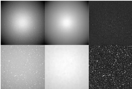
Figure 7: The original (left) image shows a high amount of vignetting. Using a minimum filter erases all details (center) which allows subtracting the background illumination from the original image to obtain a corrected image (right). While the upper row shows the complete image, the second row shows only the central part.
