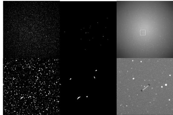
Figure 8: The binary image (left) shows many objects resulting from noise, stars and tracks. After deleting small binary objects (center) only a few binary objects are left. After measuring the properties of each object the tracks can be identified and their position measured (right).
