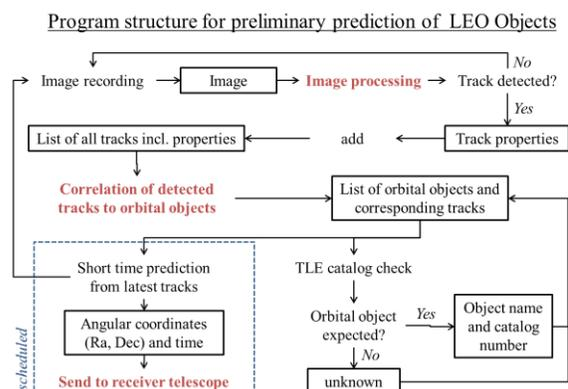
Figure 6: Overview of the program structure to detect orbital objects from continuous image recording. First tracks are extracted from image, then detected tracks are correlated to orbital object which are compared with the TLE catalogue. In future stage the system shall perform reliable predictions.
