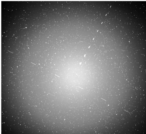
Figure 5: A composite image of 20 single frames recorded by the staring camera during a 60s observation time. Each frame has an exposure time of 1s using FLI CCD camera with Canon 135 mm f/2 lens headed to zenith. It was recorded on 17.04.2014 20:46 (UTC) and three different LEO objects passing the field of view.
