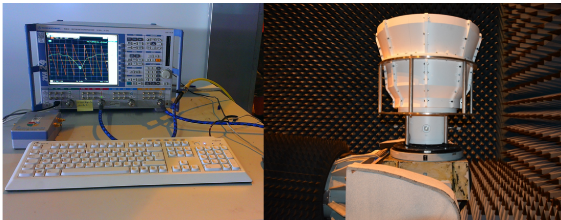
Figure 7.2: Return loss measurement: Experimental setup in DLR's Compact Test Range (CTR).
