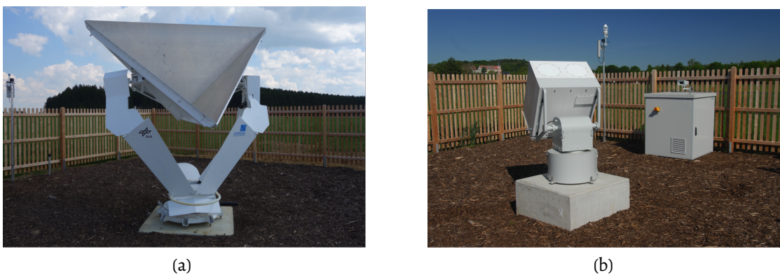
Figure 1.2: (a): DLR's first remote controlled trihedral corner reflector. (b): DLR's C-band Kalibri transponder: both designed and built for radiometric calibration and can be operated remote controlled.
