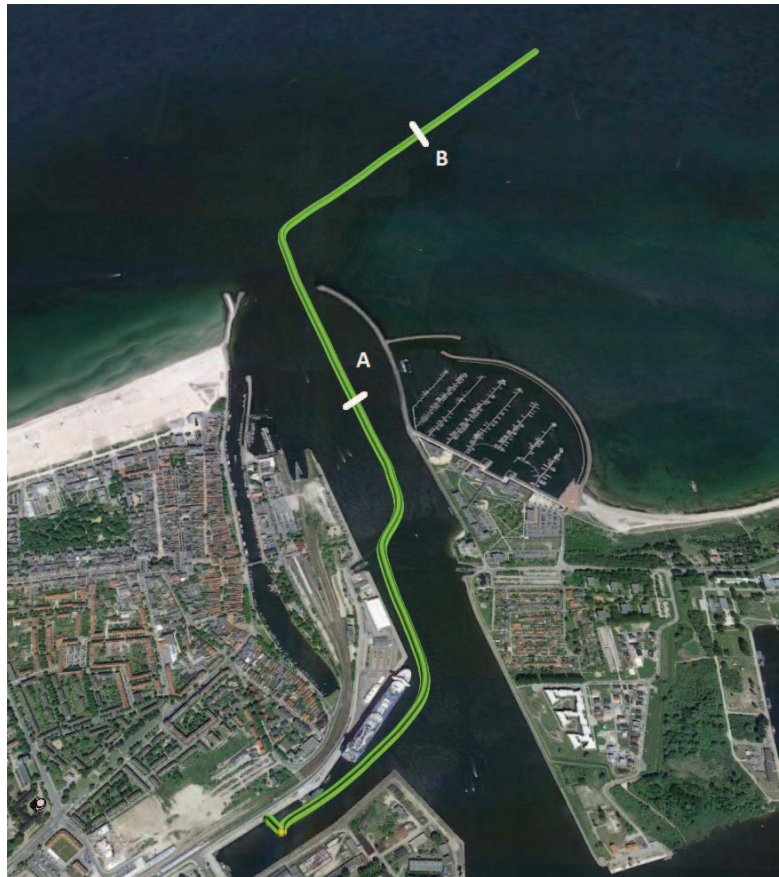
Figure 2. The test trajectory (approx. 22 min) in the port of Rostock (overlaid with the image from Google Earth). Segment AB denotes the path where GNSS signals were disabled (5 minutes).
