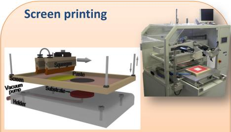
LST-GDC electrodes (Ø=16 mm) were screen printed onto YSZ pellets to obtain symmetrical cells: processing parameters adjusted to obtain 15  $\mu$ m thick electrodes. Sintering at 1100°C x 5h.
