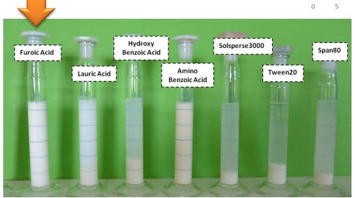
Optimization of the **deflocculant concentration** (=26 vol% in respect to the powder)
