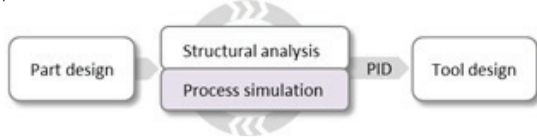
Fig. 2: A sophisticated design process considers PID as early as possible
