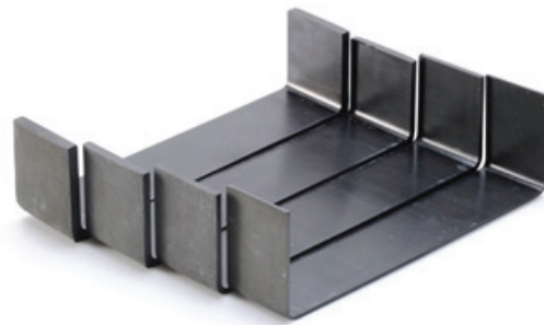
Fig.4: CFRP C-profile specimens manufactured with single-sided tool concept
