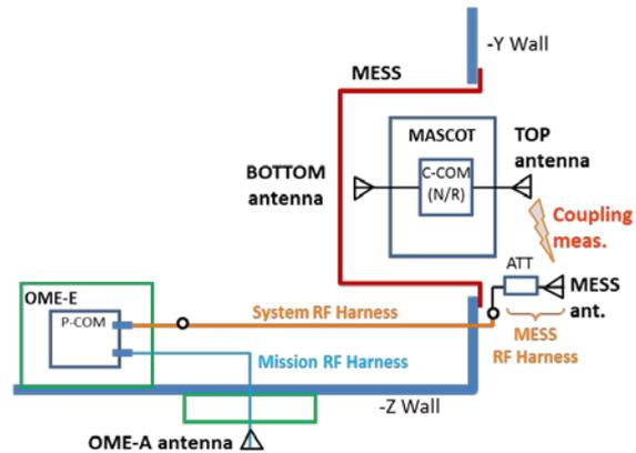
Fig. 6: RF communication chain between MASCOT and Hayabusa2
