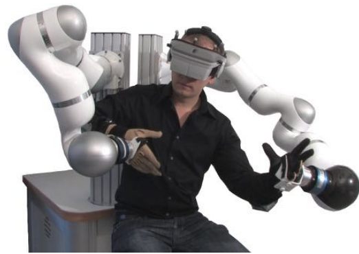
Figure 10. The bimanual haptic device HUG of the DLR provides the human operator with force feedback from the virtual world. Magnetic clutches couple the human hands safely to the robots, while data gloves determine the finger positions.
