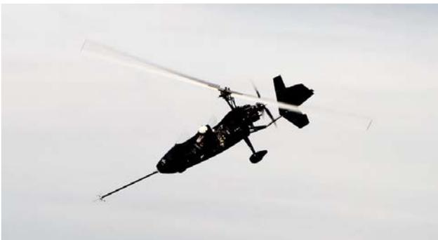
Figure 6: *MTOsport gyroplane with special flight test instrumentation during flight test*
