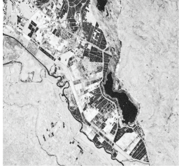
Fig. 3. As an example of the coherence response of flooded agricultural fields in TanDEM-X images, making the segmentation of the fields very precise.
