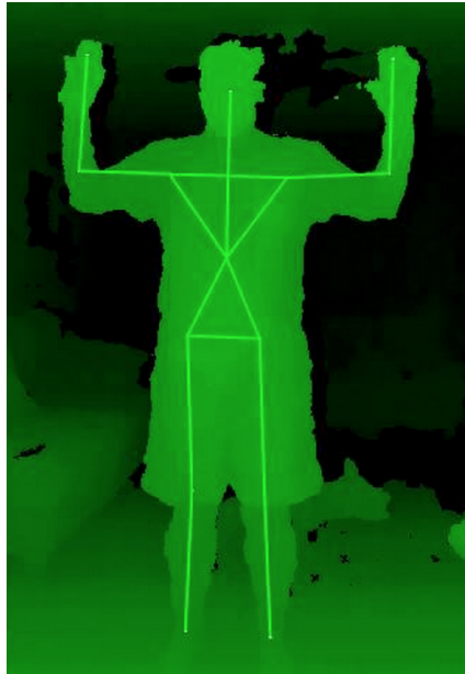
Figure B.3: Skeleton and depth image provided by Kinect.
