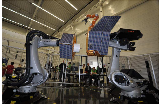
Fig. 1: Overview of the OOS-SIM. Left: Client satellite; Right: Servicer satellite and manipulator
