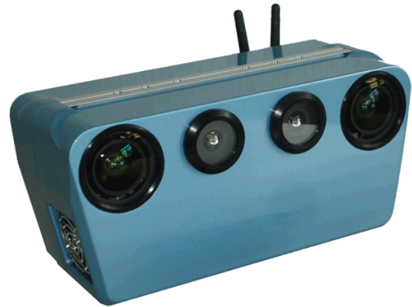
Figure 1: IPS sensor head, stereo cameras (left and right) and the lighting system (middle) can be seen. Dimensions: about 30 x 15 x 10 cm 3 , Weight: about 4kg, depending on configuration
