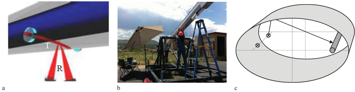
Fig. 1 (a) Optical path of transmittance and reflectance measurement at CENER [2] (b) Calorimetric outdoor test bench at NREL [6] (c) Scheme of linear focus solar simulator receiver test bench at DLR
