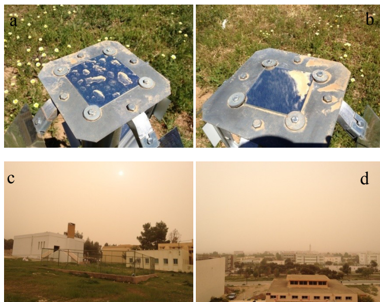
Fig. 2. Dust deposition on horizontal mirror surfaces after a sand storm. (a) Dust deposition on aluminum mirror; (b) Dust deposition on a 4 mm thin glass mirror; (c-d) Photo showing the high aerosol concentration in the atmosphere during a sand storm in Oujda City.
