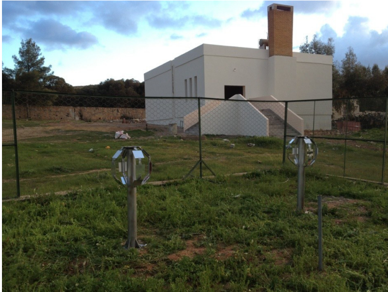
Fig. 1. Stand-alone mirror spheres installed at the University of Oujda.
