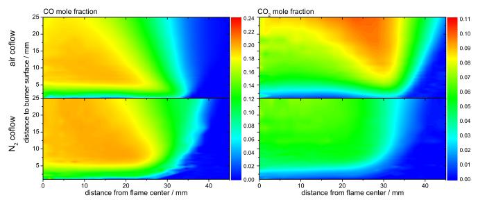
Fig. 5 Mole fraction maps of CO (left) and CO<sub>2</sub> (right) in the investigated fuel rich methane/oxygen ( $\phi = 1.6$ ) flame with air (top) and N<sub>2</sub> (bottom) coflow gas.
