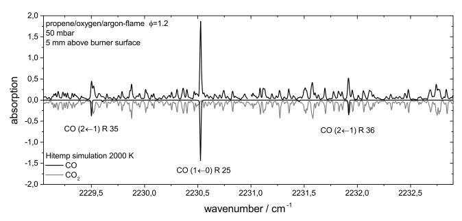
Fig. 3 Absorption spectrum of CO and CO<sub>2</sub> measured in a fuel rich propene flame at 50 mbar around  $4.48 \,\mu\text{m}$ . The simulated spectra of both molecules are plotted on an inverted scale.
