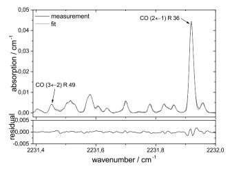
Fig. 4 Abel-inverted absorption spectrum of CO and CO<sub>2</sub> in a fuel rich ( $\phi = 1.6$ ) methane/oxygen flame at 50 mbar and corresponding fit based on the constants from the HITEMP database. The two lines of CO in this region are marked with arrows; all remaining lines are due to CO<sub>2</sub>.
