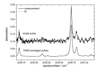
Fig. 8 Single-pulse and averaged absorption spectra together with the fitted spectrum. Measurements were performed in a gas cell at  $178\,\mathrm{mbar}$  and  $294\,\mathrm{K}$  at a laser repetition rate of  $20\,\mathrm{kHz}$ . The single-pulse spectrum has been shifted for clarity.
