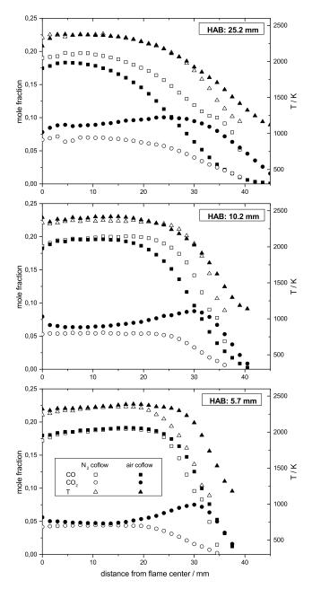
**Fig. 6** Radial profiles of temperature, CO and CO<sub>2</sub> mole fractions for different heights above the burner (HAB) in a fuel rich methane/oxygen ( $\phi = 1.6$ ) flame. Open symbols: With N<sub>2</sub> coflow. Closed symbols: With air coflow.
