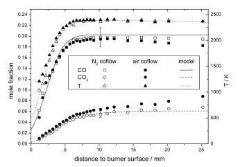
Fig. 7 Flame center mole fraction and temperature profiles in the investigated fuel rich methane/oxygen ( $\phi = 1.6$ ) flame with different coflow gases. Model simulations were performed with ChemkinII and the GRI3.0 mechanism.
