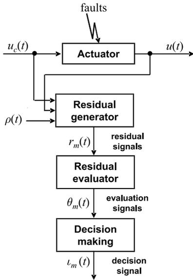
Fig. 1. FDD system for parametric LOE monitoring.
