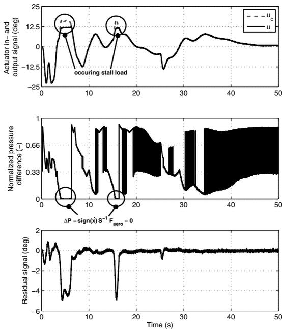
Fig. 5. Stall loads during a high input maneuver.
