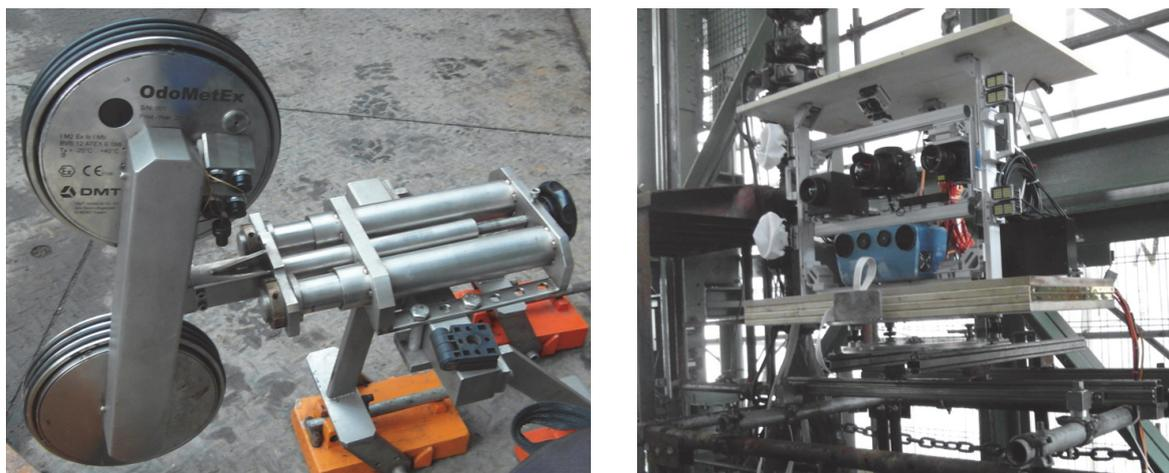
Figure 4: Odometer (DMT) before installed inside the pit cage (left). Installation of the test setup on top of the pit cage. The PCO camera used for this evaluation is the most right of the three black cameras (right)
