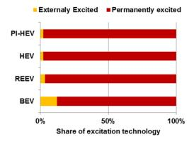
Figure 7: Share of excitation technology per electrification concept
