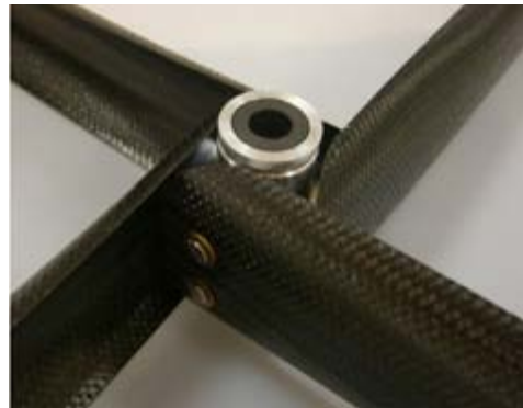
Figure 2-4: Four C-shaped bi-stable booms attached to the central hub of the GOSSAMER DEORBITER [4].
