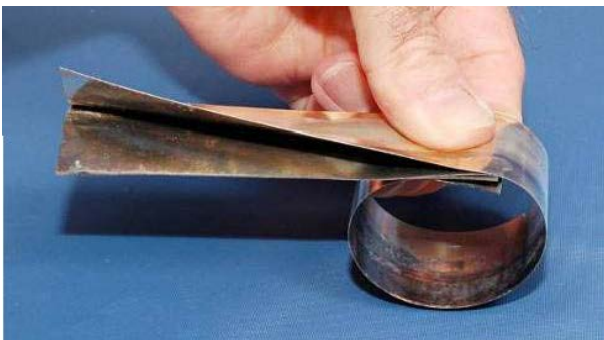
Figure 2-2: Folding of a TRAC boom sample [7].
