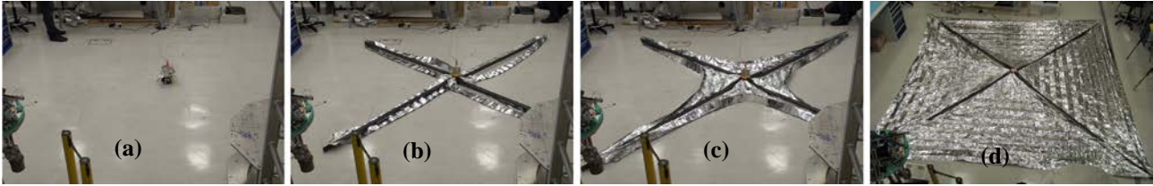
Figure 3-1: Deployment sequence of the DE-ORBIT SAIL engineering model: (a) fully stowed, (b) prior to in-plane opening of the sails, (c) sail opening and (d) fully deployed.
