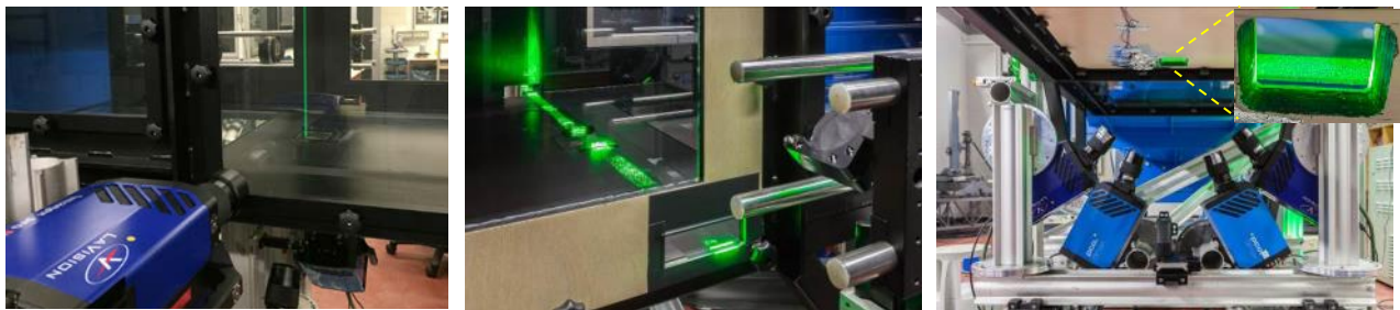
Figure 1: Left: Imaging setup for boundary layer profile measurements by high-repetition-2C-PIV in the 1m-Wind Tunnel of DLR Göttingen. Middle: Collimated laser light volume with passe-partouts parallel to the wall Right: In-line camera high-repetition STB set-up with four PCO Dimax-S4 cameras viewing through a glass insert of the wall.
