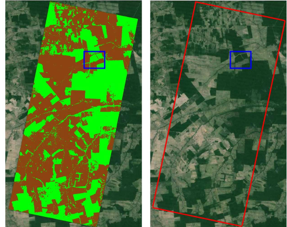
Fig. 5. Forest/non-forest classification map (depicted in green and brown, respectively) of an area located in the Amazon rainforest, Brazil, overlaid on a GoogleEarth optical image, which is given on the right-hand side for comparison. The considered area is delimited by the red rectangle and extends by about 55 \text{ km} \times 30 \text{ km} .
