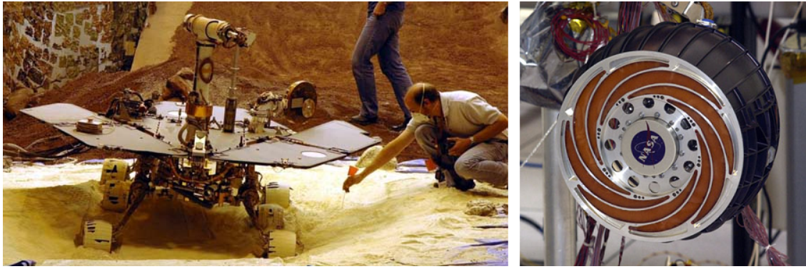
Figure 2.6: Left: Researchers at JPL simulate the conditions faced by the rover Spirit on Mars, where it was stuck in loose soil, to find the best way to help free it. Right: MER wheel. (Courtesy NASA/JPL-Caltech)
