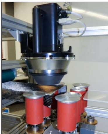
Figure 9. Forming unit with FScan sensor for fiber orientation measurement
