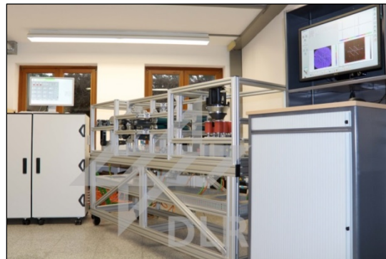
Figure 6. DLR continuous profile preforming line
