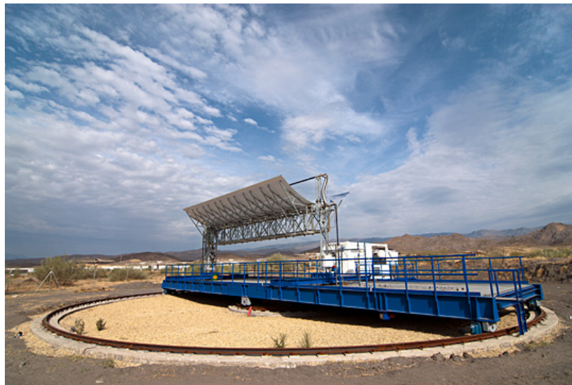
Figure 4.3: Side view of KONTAS rotary test bench
