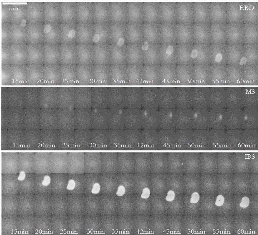
Figure 3: Fluorescence micrographs after LIC tests show deposit formation. Laser irradiation time varied from 15 min up to 60 min. Fluence was 300 mJ/cm<sup>2</sup> with contamination pressure of  $2 \times 10^{-5}$  mbar.
