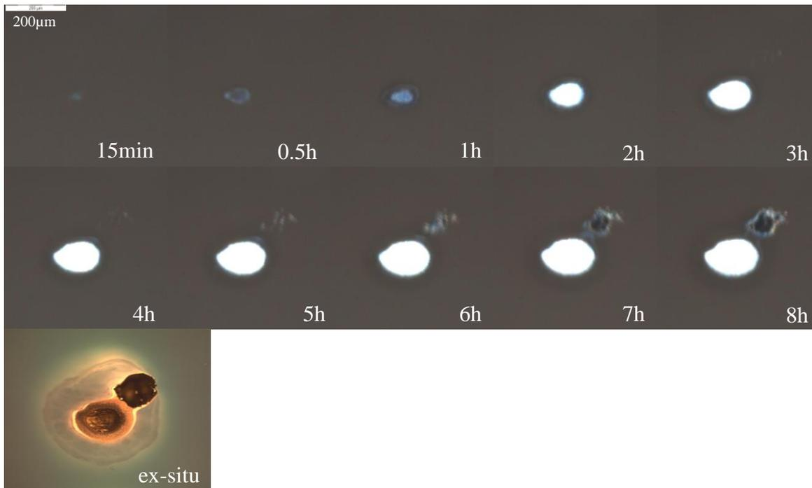
Figure 9: In-situ long distance microscope images of IBS sample during LIC test and ex-situ DIC micrograph made after the test. Sample tested at a fluence of 360 mJ/cm<sup>2</sup> and a contamination pressure of 3.5 x10<sup>-5</sup> mbar.
