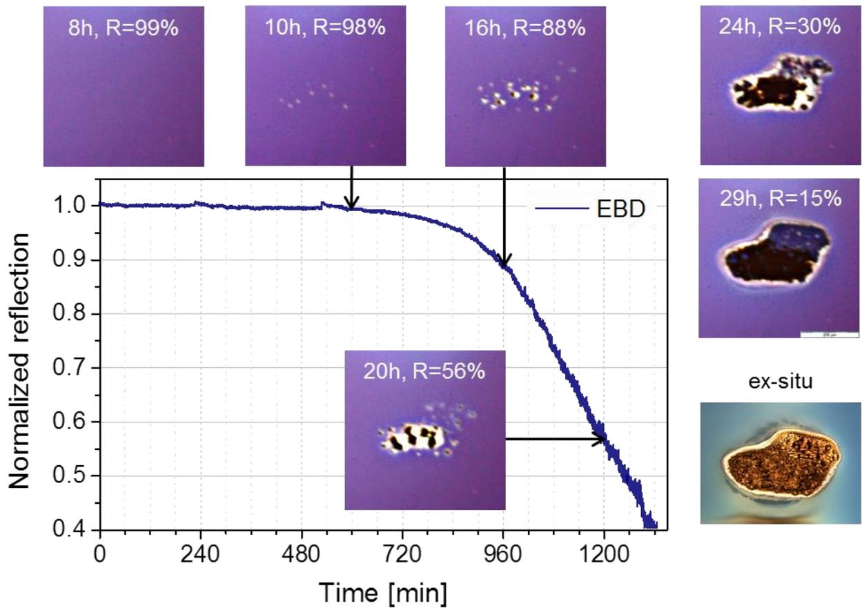
Figure 7: Normalized reflection measurement of the EBD sample during a LIC test. Test conditions are  $H_{\text{Peak}} = 400 \text{ mJ/cm}^2$  with a contamination pressure of  $p = 3.1 \times 10^{-5} \text{ mbar}$ . After 10 h (36 mio. shots) of irradiation the reflection starts to degrade and in-situ long distance microscope images show damage growth. In addition ex-situ DIC micrograph is shown.
