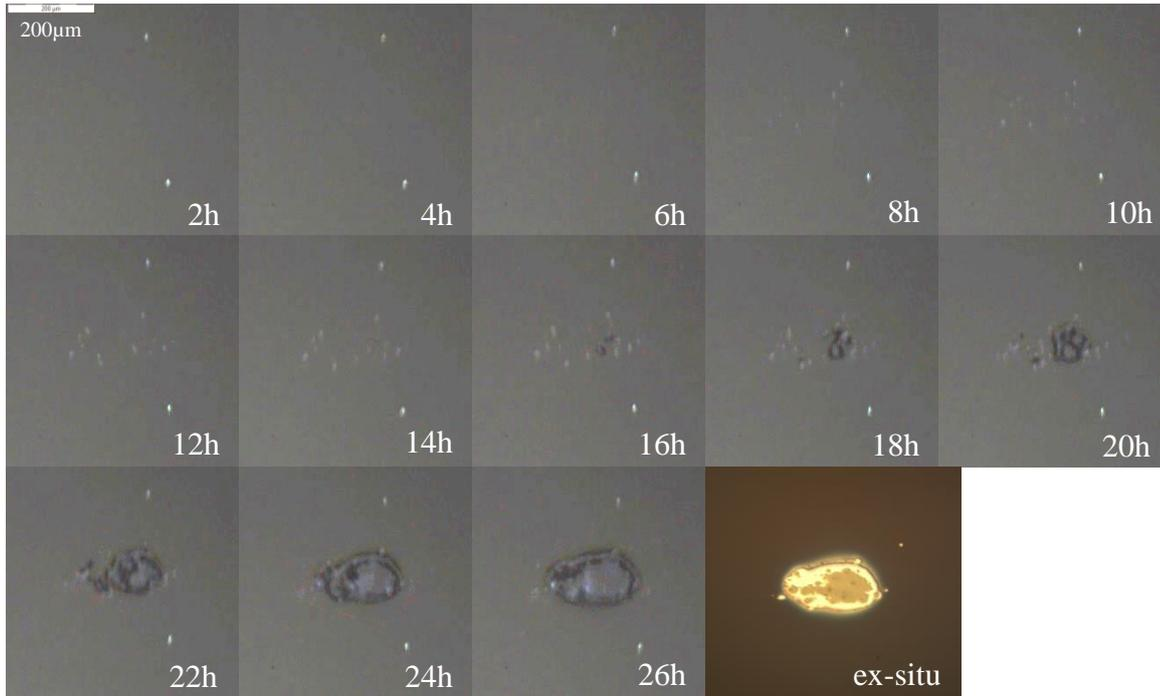
Figure 8: In-situ long distance microscope images of MS sample during LIC test and ex-situ DIC micrograph made after the test. Sample tested at a fluence of  $660 \text{ mJ/cm}^2$  and a contamination pressure of  $1 \times 10^{-5} \text{ mbar}$ .
