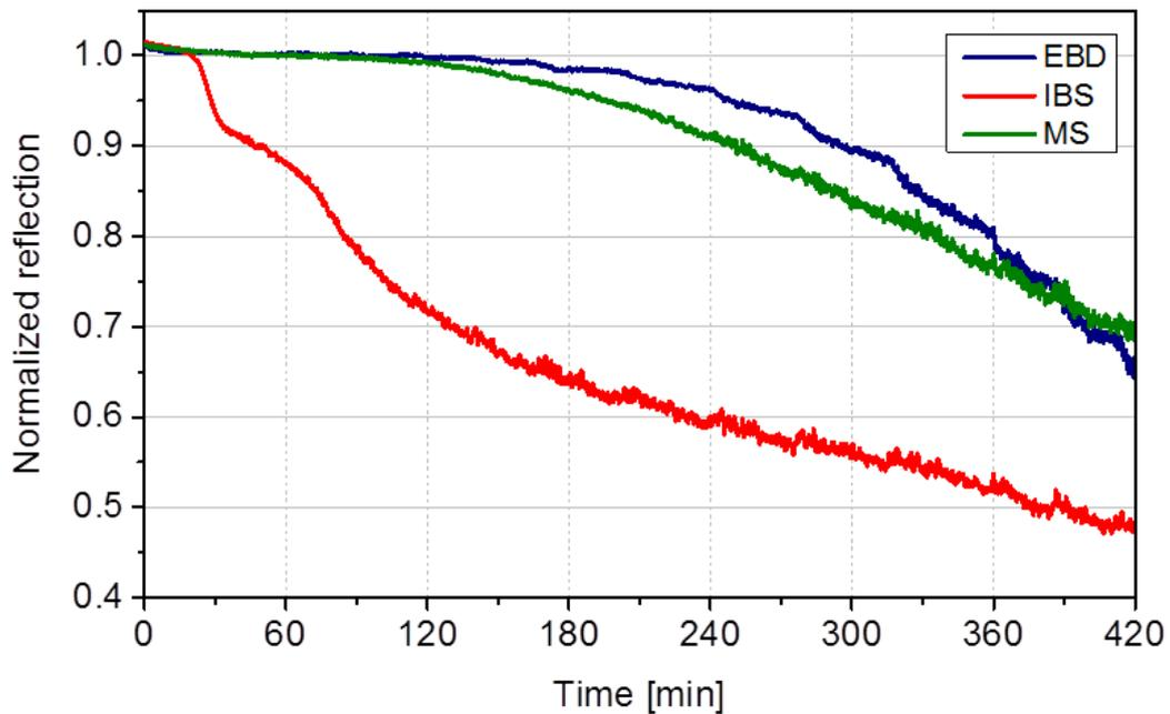
Figure 5: Normalized reflection measurement of the EBD, MS and IBS samples during a LIC test. Test conditions are  $H_{\text{peak}} = 900 \text{ mJ}/\text{cm}^2$ , with a contamination pressure of  $p = 4 \times 10^{-5}$  mbar.
