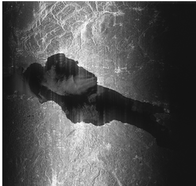
Figure 9. Focused image acquired by the German satellite TerraSAR-X in staggered SAR mode over the Lake of Constance. The azimuth sidelobes visible in the Lake of Constance are from strong scatterers, since it was not possible to use an optimum nonuniform PRI sequence due to TerraSAR-X commanding restrictions.
