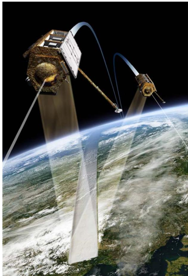
**Fig. 1:** TSX and TDX satellites flying in close formation. With across-track baseline values ranging from 120 to 500 m a high-resolution global Digital Elevation Model is being generated.
