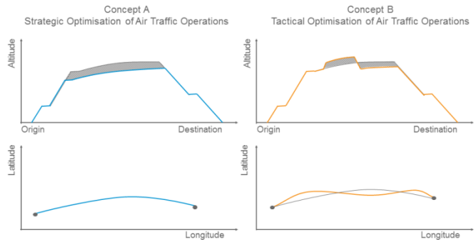
FIG 11. Strategic, climate-dependent optimisation of air traffic (left; same change in flight trajectory is performed every day) vs. tactical, weather-dependent optimisation (right; different flight trajectories for every day). The thin black lines represent the reference trajectories with minimal costs.
