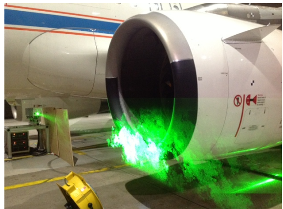
Figure 10: Laser under fuselage with outboard directed light sheet in front of the blackened engine inlet lip
