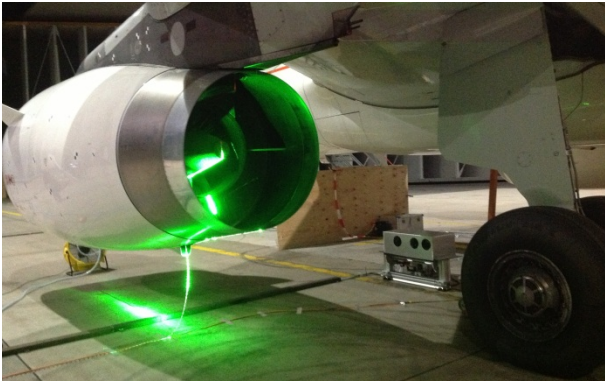
Figure 4: Laser light sheet from behind engine hitting the core plug with diffuse reflection
