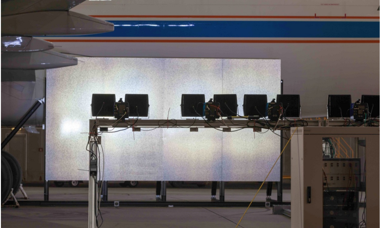
Figure 15: Retro-reflexive background with random dot pattern and four 4 Mpx PCO Dimax high-speed cameras with each two lateral pulsed and collimated LED-arrays
