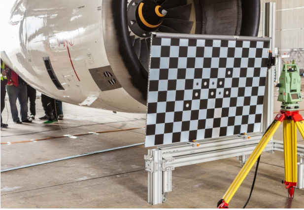
Figure 12: Calibration target with checker board having an inclination angle of 6° and blackened engine inlet lip
