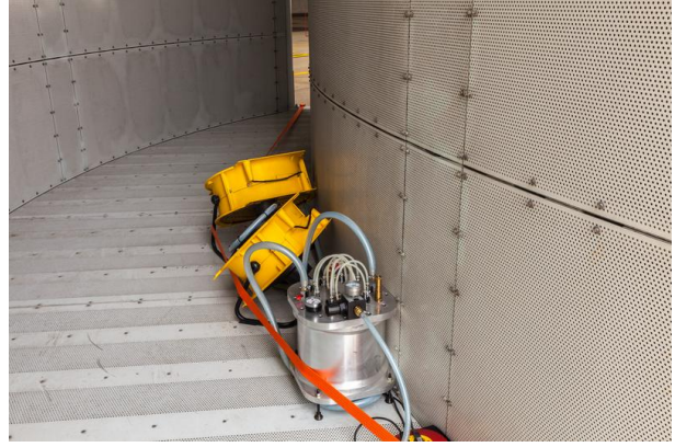
Figure 13: Particle generator and blowers between airflow guide vanes in the gate
