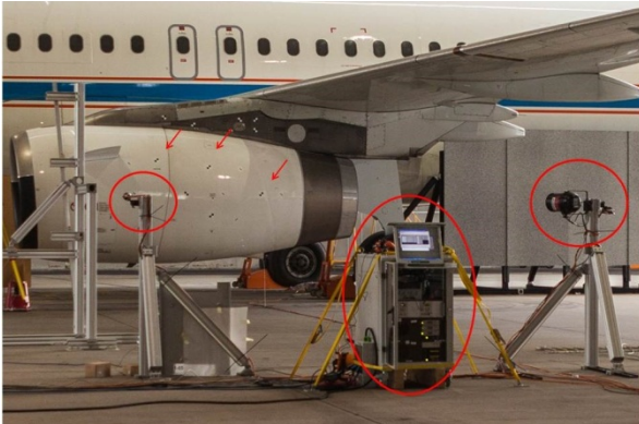
Figure 7: MODE system; in front two supports with cams and LED lamp (circles), DAQ centered (ellipse); in background: nacelle with reference markers (arrows)
