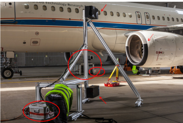
Figure 9: PIV system with laser in the back (circle); cameras in casings in front (arrows); aluminum boxes as electronic safety boxes (ellipses)
