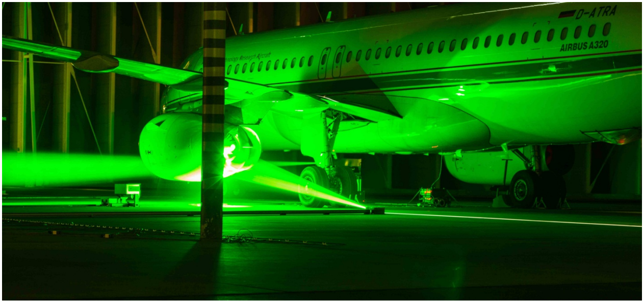
Figure 14: Laser light sheets at the ATRA V2527 engine for measuring SPIV in the engine inlet and the bypass jet exit flow during operation at MCT in the sound-attenuating hangar of the airport Hamburg
