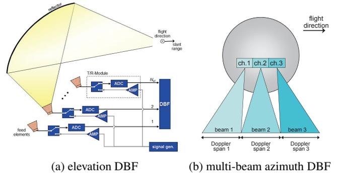
**Fig. 1:** Conceptual system architecture for digital beamforming (DBF) operation.
