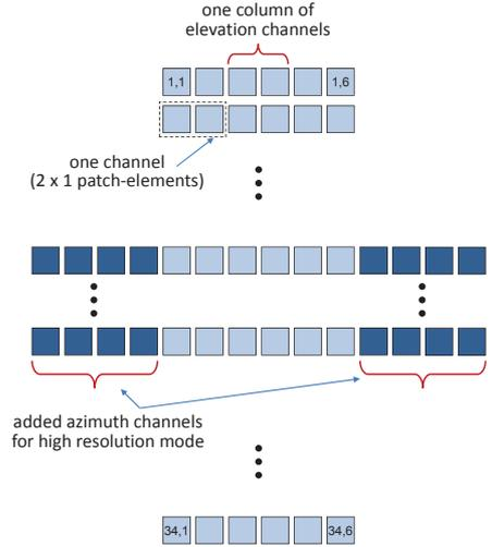
Fig. 2: Patch arrangement for the digital feed antenna.
