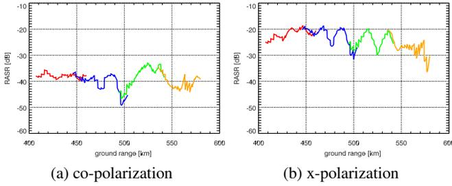
**Fig. 5:** range-ambiguity-to-signal ratio of co- and X-pol of mode B4
