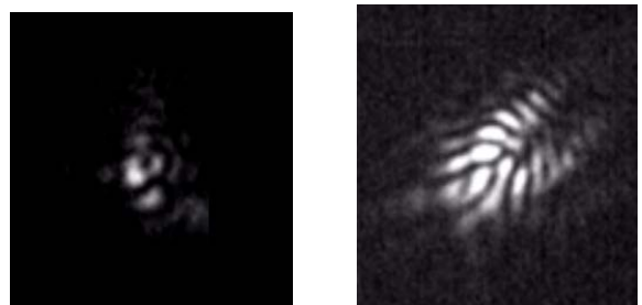
Fig. 6. Example of a small focal speckle pattern due to a large Fried parameter (left), and a bad IRT-situation, causing a large focal speckle pattern (right); measured during EFAL Antarctic r_0 measurement campaign Dec'13-Feb'14.
