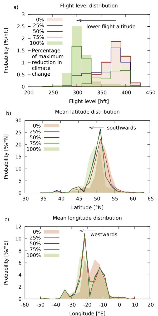
**Fig. 5.** Change of the probability density function of air traffic characteristics along the Pareto front for westbound air traffic and P-AGWP100. a) flight level, b) mean latitude and c) mean longitude. See also Supplementary information (Fig. S3) for the interpretation of mean longitudes and latitudes.
