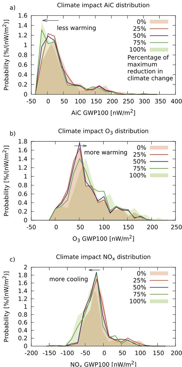
**Fig. 8.** Change of the probability density function of air traffic characteristics along the Pareto front for westbound air traffic and P-AGWP100. a) Contrail b) ozone c) NO<sub>x</sub>.
