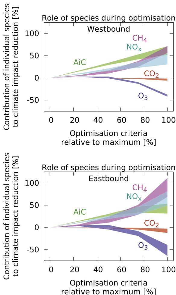
**Fig. 9.** Contribution in [%] of CO<sub>2</sub> (red), contrails (AiC, green), ozone (blue), methane (magenta), and total NO<sub>x</sub> (=O<sub>3</sub> + CH<sub>4</sub> + PMO) to the climate warming reduction by re-routing the North-Atlantic air traffic. The area between the minimum and maximum values for all metrics is highlighted.
