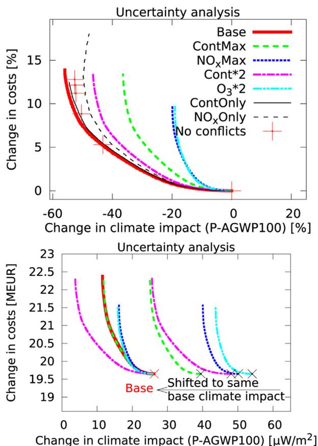
**Fig. 10.** Pareto front for westbound air traffic P-AGWP100 (analogously to Fig. 3) for various sensitivity analyses (see Table 4). Top: relative numbers in [%]. Bottom: Absolute changes in [MEUR] and [ $\mu\text{W m}^{-2}$ ].
