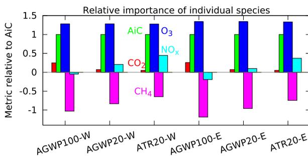
**Fig. 4.** Relative importance of individual species for a reduction of the climate impact for air traffic. For each metric and direction (see also Fig. 3) the change in the metric value for  $\text{CO}_2$  (red), contrails (AiC, green), ozone (blue), methane (magenta), and total  $\text{NO}_x$  ( $\text{O}_3 + \text{CH}_4 + \text{PMO}$ , cyan) are given relative to the respective value for contrails (hence contrails are always 1).
