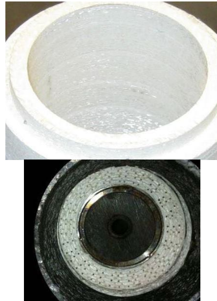
Figure 13: WPS oxide CMC ring segment of a 50 mm model combustor (top), additionally implemented injector channel patterns (bottom)
