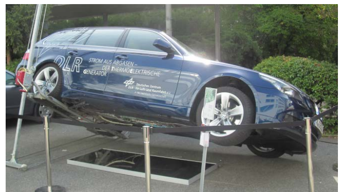
Fig.16: Test platform with thermoelectric generator in the exhaust system based on a BMW 5series
