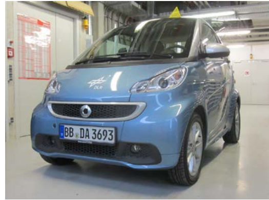
Fig. 12: Test platform for fuel cell range extender based on an electric Smart vehicle
