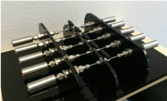
Fig. 14: Coupled thermochemical storages to produce heat and coldness at the same time
