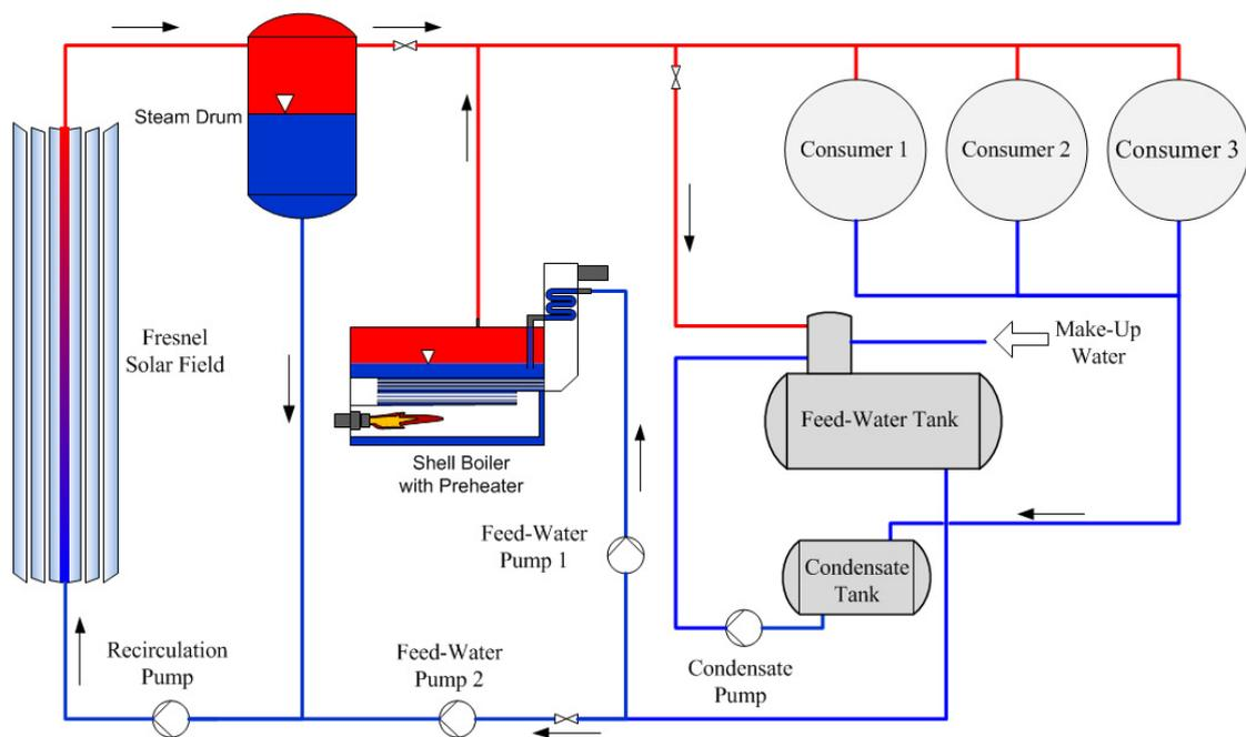
Figure 5: Proven layout for solar process heat integration in conventional steam circuit
