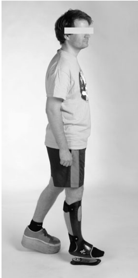
Figure 1 HEPHAISTOS. A subject wearing the HEPHAISTOS unloading orthosis and the elevated contralateral plateau shoe.
