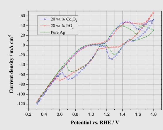
A mixture of silver and 20 wt.% Co<sub>3</sub>O<sub>4</sub> or IrO<sub>2</sub> shows the highest current densities. Also potentiostatic polarization curves show enhanced current densities and a stable behavior after 200 s for ORR and OER. Especially the combination  $Co_3O_4$  and silver shows also an excellent long-term stability over 200 cycles. Impedance spectra shows that total resistances in ORR and OER of the electrodes correlate to the achieved current densities [2].
