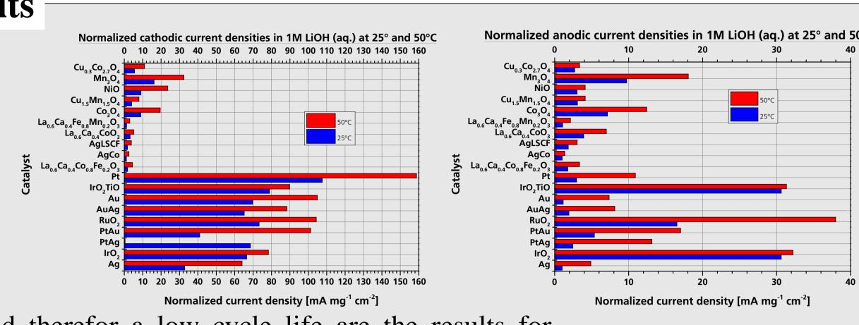
Batteries. A high degradation and therefor a low cycle life are the results for carbon based electrodes. This work shows carbon-free electrodes consisting of metal and metal oxides exhibiting high current densities at relatively low overpotentials and a high cycle life (< 200 cycles) [2].
