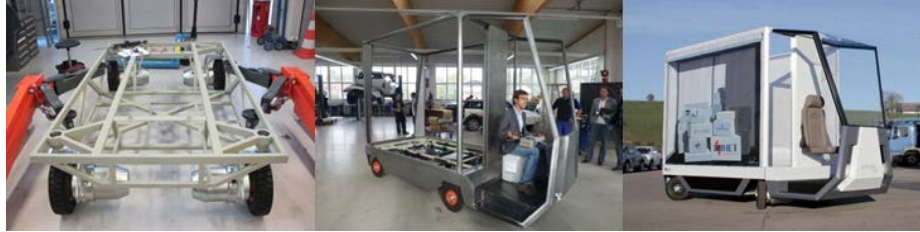
Fig. 9: Example development of a prototype construction
