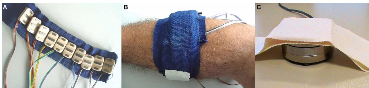
**FIGURE 1 |** The setup of the first experiment. (A) Ten OttoBock MyoBock 13E200 sEMG electrodes, uniformly arranged (B) on the subject's forearm using a band of bio-compatible adhesive tape. (C) An ATI Mini45 force sensor, kept in place using double-sided tape.
