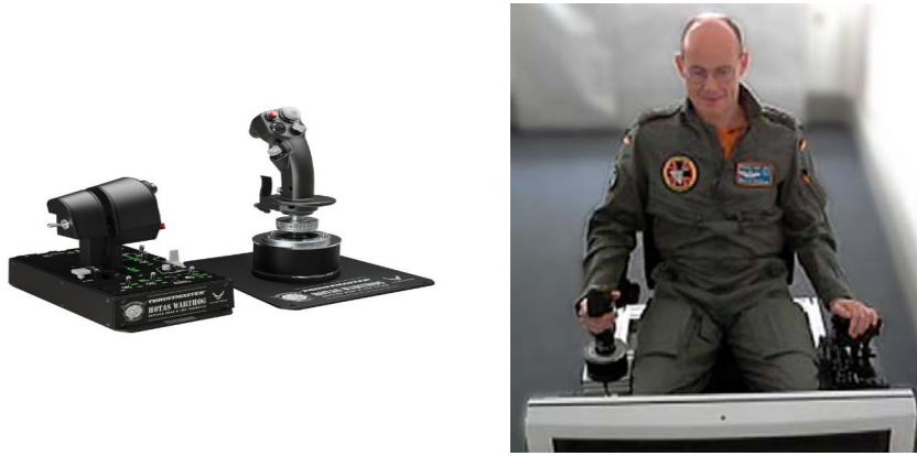
Figure 3-2: Thrustmaster HOTAS Warthog Hardware and Simulator Setup with Test Pilot
