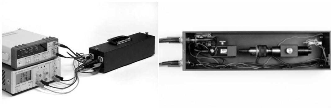
Fig. (4). Photomultiplier clinostat (black box), frequency counter and power supply (left) and details (PMT, cuvette, motor) (right).
