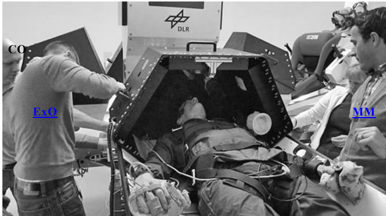
Fig. (3). Short Arm Human Centrifuge (SAHC) Subject in preparation for the run by the Medical Monitor (MM), the Experiment Operator (ExO) and the Centrifuge Operator (CO).
