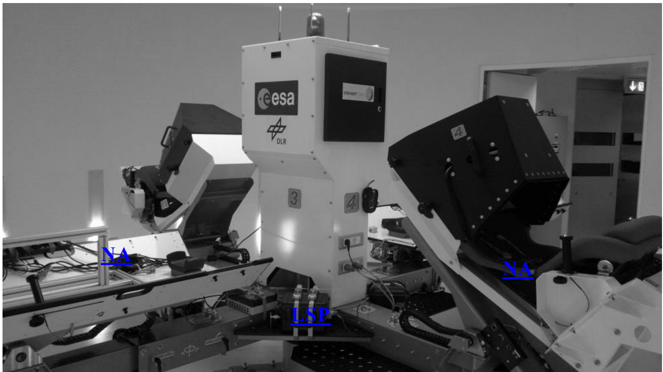
Fig. (2). Short Arm Human Centrifuge (SAHC), Life Science Platforms (LSP) and nacelles (NA) of the SAHC.
