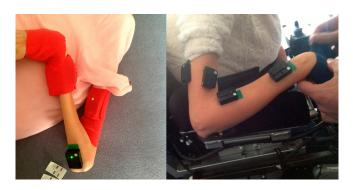
Fig. 3. Electrode placement for subject SH (left) and SV (right). Electrodes are fixed with doublesided medical tape and additionally wrapped with medical cohesive tape to ensure fixation (left).
