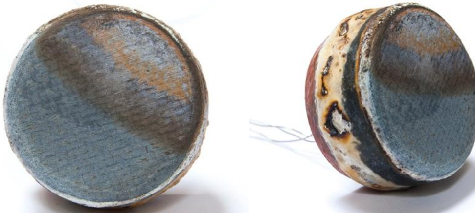
Figure 22. Sample C/C-1 after test 16. There was a certain amount of oxidation in the upper region of the sample where the hot spot had formed multiple times. The coating on the circumference was performing well and it was possible to re-apply it between tests.
