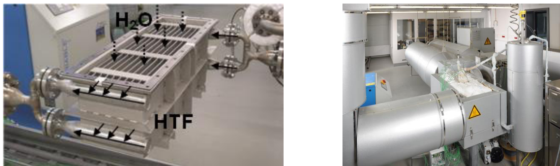
Fig. 1. Left: Indirectly operated thermochemical storage reactor (top cover not shown); Right: Picture of multifunctional test bench
