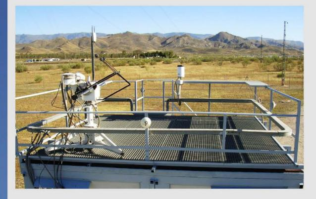
The main interests of the solar radiation characterization at PSA are to analyze relationships between solar variables, to assess low-cost atmospheric attenuation devices, to improve estimations from satellite images, to analyze the spectral distribution of solar radiation under different conditions, and to test the international standards for the calibration of solar irradiance sensors.
