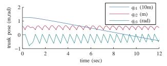
Fig. 9. Time evolution of the trunk pose for the forward hopping motion. The coordinates  $q_{t_1}$  and  $q_{t_2}$  represent the horizontal respectively vertical position and  $q_{t_3}$  the orientation of the trunk.
