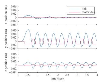
Fig. 4. Results of the hitting experiment. The plots depict the motion of the end-effector and the time evolution of the desired motor positions in terms of end-effector positions. Both representations refer to the coordinate system fixed to the ground, displayed in Fig. 3.
