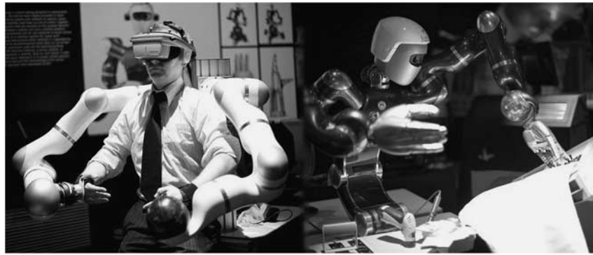
Figure 1 Demonstration of robotic on-orbit servicing using a tele-presence interface (left) to control a humanoid robot and manipulate a physical satellite mock-up (right).
