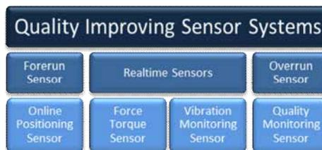
Figure 4: Quality improving sensor systems for the fibre placement process
