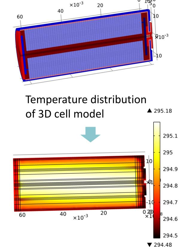
3D simulation is compared with 1D simulation under nominal discharge operation in 1 hour (1C rate).
