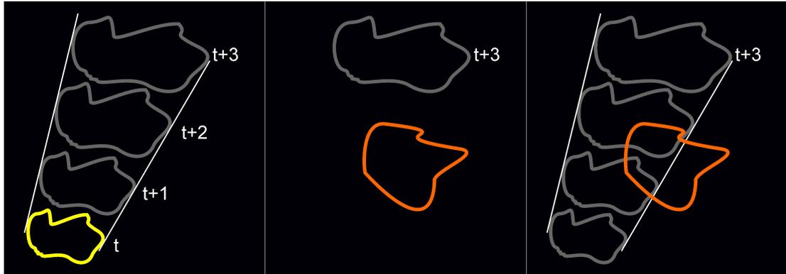
**Figure 4.3.:** Left: Cb-TRAM CI detection at time step  $t$  (yellow contour) with its nowcasts for the next three time steps  $t+1$ ,  $t+2$  and  $t+3$  (gray contours). Middle: Time step  $t+3$  with the corresponding nowcast of the CI cell (gray) and a new stage 2 detection nearby (orange). Right: Time step  $t+3$  with its "nowcast track" (all older positions of this detection in gray) now overlapping with the nearby detection.
